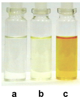
Figure 4. Color changes observed: (a) receptor 1 , (b) on addition of benzoate and (c) on addition of fluoride.
